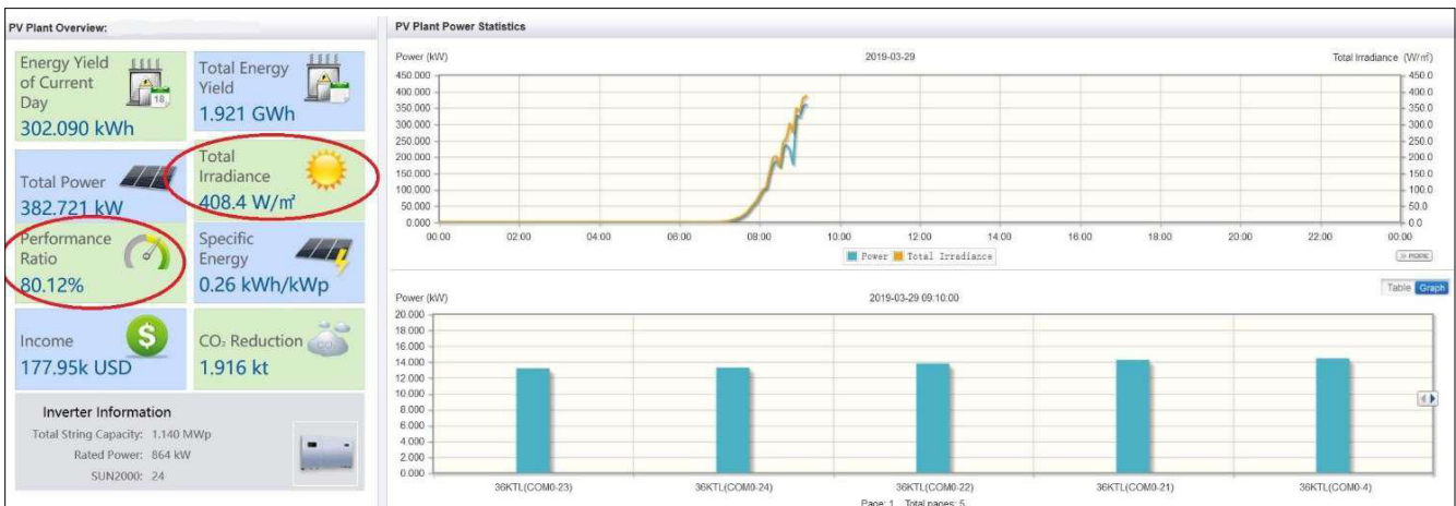
Figure 7: NetEco Monitoring System
